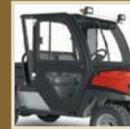
ROPS Cab (Roll Over Protective Structure)
